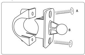
Step 3. Wrap the rubber rings (C) around the handlebar and reassemble the 17mm ball plate (B) around the rubber rings. Secure the mount assembly by using the screwdriver to retighten the two mounting screws.
