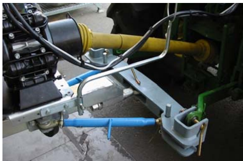
Tractor coupling for homologated Towed machines in work position (not suitable for road use).
