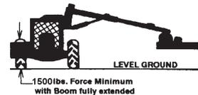
If the unit is operated on slopes greater than 5°, additional counterweight will be required. Operation of the unit on slopes greater than 11° is not recommended under any circumstances. On a tractor with a 96" outside to outside tire spread, a 11° slope occurs when one rear tractor tire is about 8" lower than the other rear tire.
