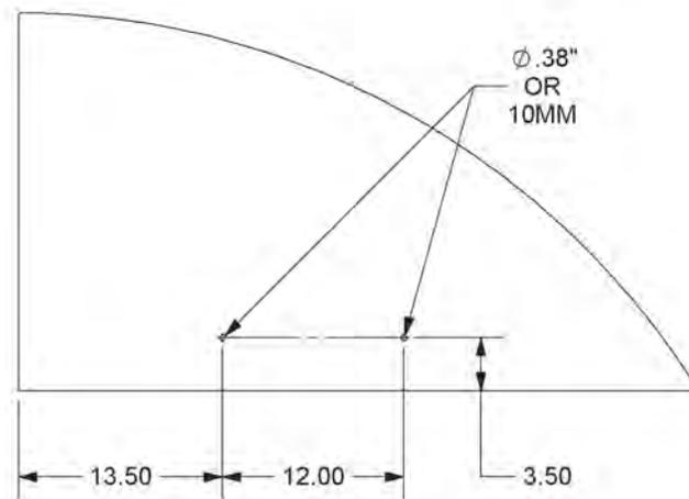
Place as many hoses in the clamp that will fit without compromising pressure. Then secure the (2) HOSE CLAMP (06520013) to the holes drilled with (1 EACH) CAPSCREW, 3/8" X 1", NC (21630) and (1 EACH) NYLOCK NUT, 3/8", NC (21627). The hoses that don't fit into the clamp are to be secured to the others with zip-ties. For protection of hoses in contact with metal edges, wrap hoses with spit hose sections and fasten with hose clamps or zip ties as needed.
