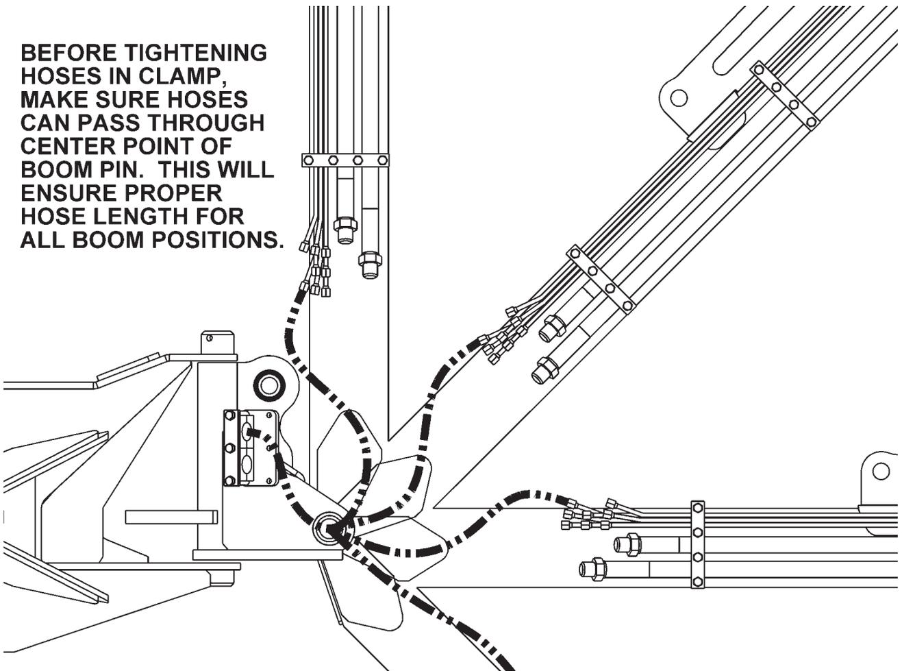
Arrange the hoses in the clamp that attaches to the boom mounting bracket as shown above, with the 1" motor hoses closest to the bracket and the return hose closest to the boom arm. Pull the hoses snug from the swivel to the mounting bracket clamps, when main boom is still forward, and tighten the hoses in the clamp.
