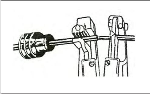
1. Apply seal to cable, before stripping insulation.
