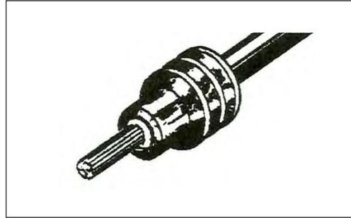
2. Align seal with cable insulation.
