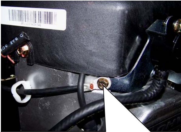
Negative battery ground on ZT2350
