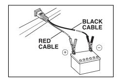
For charging 12 voltage battery, 12V-8.3A (100W) of maximum AC power can be taken out from the DC receptacle by means of the exclusive DC cable.
