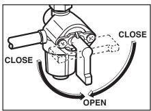
(d) Set choke lever to close if the engine is cold.
