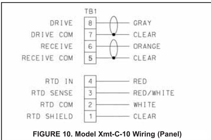
FIGURE 10. Model Xmt-C-10 Wiring (Panel)
