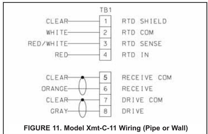
FIGURE 11. Model Xmt-C-11 Wiring (Pipe or Wall)
