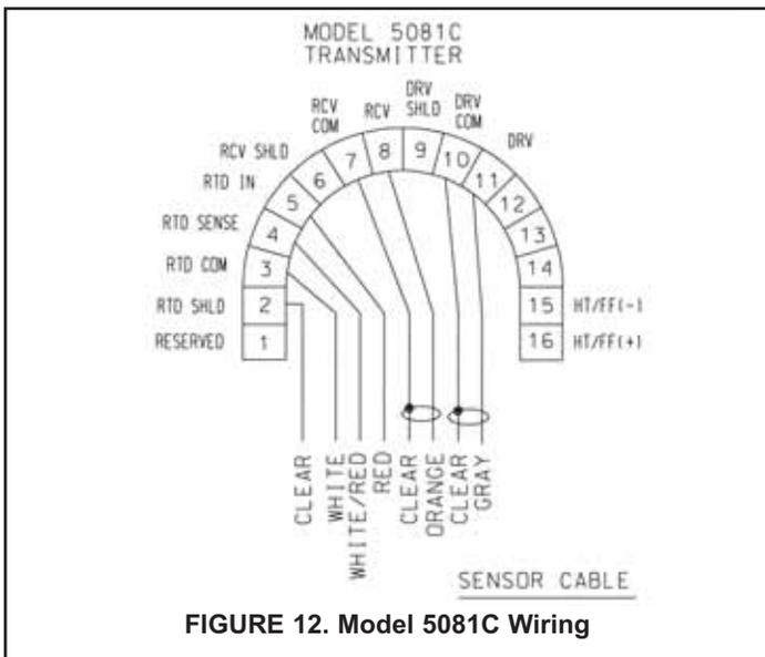
FIGURE 12. Model 5081C Wiring
