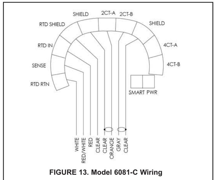
FIGURE 13. Model 6081-C Wiring
