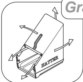
Raise the rear deflector and lift the grassbag through the handlebar and lower the rear deflector to rest against the rear of the mower.
