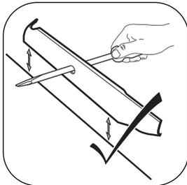
Ensure that the cutterblade is balanced. Use a screw driver with a round shaft to support the cutterblade through its centre hole. Hold the cutterblade horizontal and then release. A balanced cutterblade will remain horizontal.
