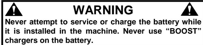
5. Slow charge the battery at 1 amp for 2 hours to bring the battery to full charge.
