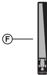
F. Reverse Speed. Shows reverse speed operation (manual drive models). Refer to Operation section.
