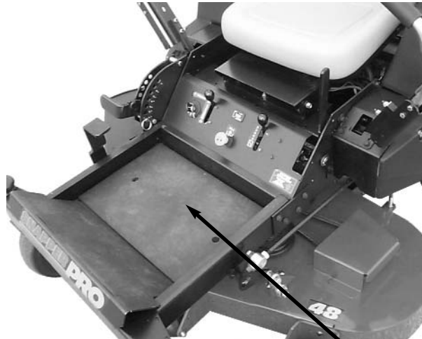
LIFT FOOT REST UP AND OFF POWER UNIT FRAME TO GAIN ACCESS TO MOWER BELT
