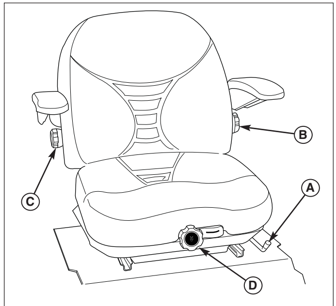
Figure 28. Suspension Seat Adjustment A. Forward / Backward Seat Adjustment Lever B. Lumbar Adjustment Knob C. Back Angle Adjustment Knob D. Suspension Adjustment Knob
