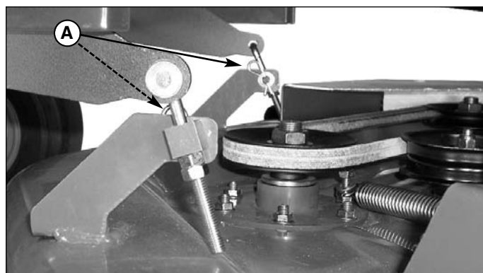
Figure 12. Front Deck Lift Components A. Hairpin Clip & Washer (Right side shown, left side hidden)
