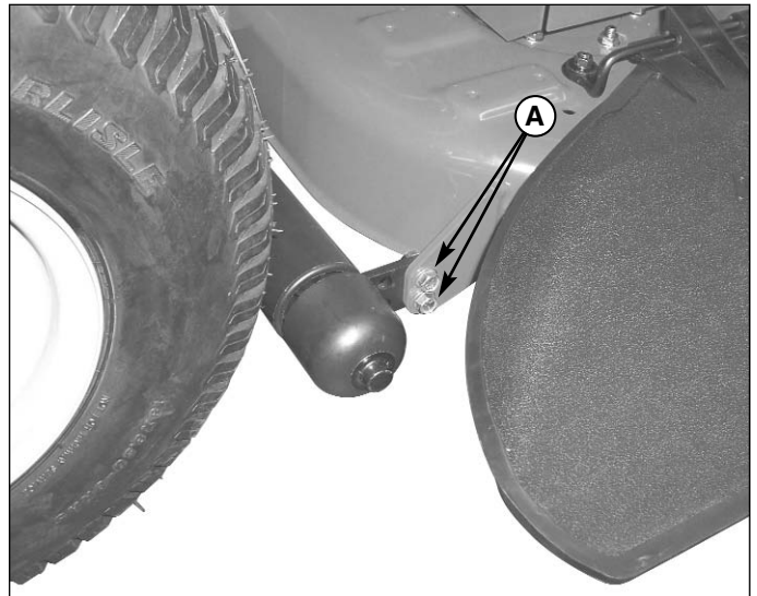
Figure 32. Roller Bar Leveling A. Leveling Hardware
