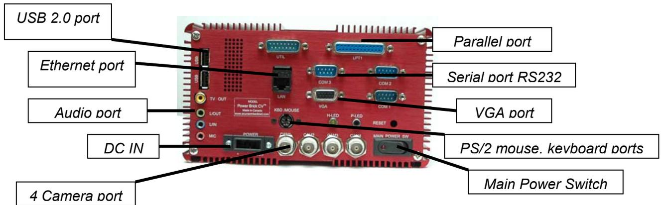
**Figure2.2: Back side of PowerBrick-CV.**
