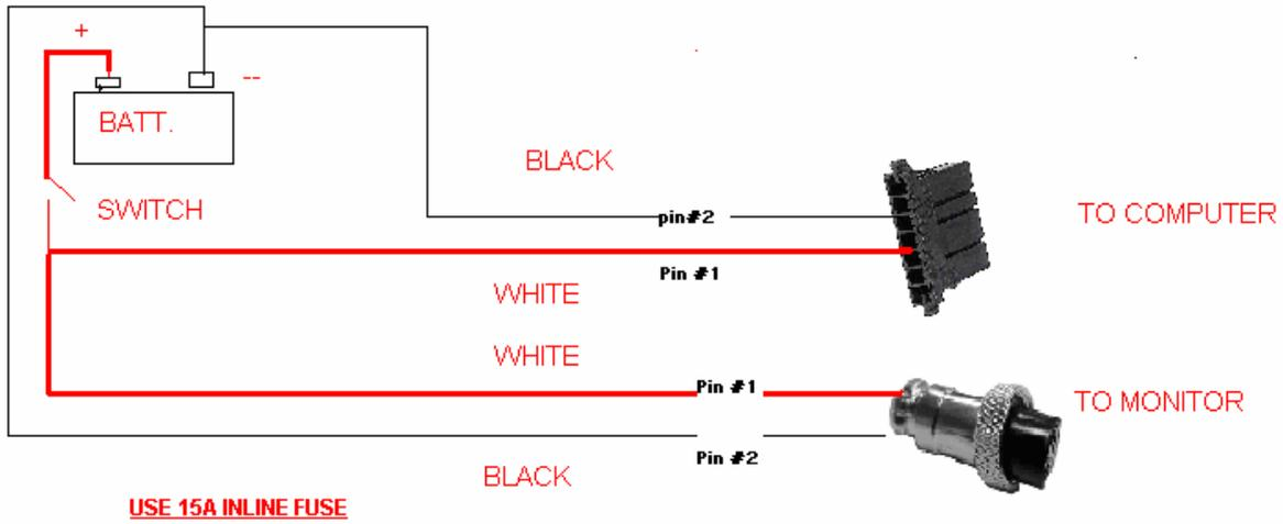
POWER BRICK WIRING DIAGRAM
