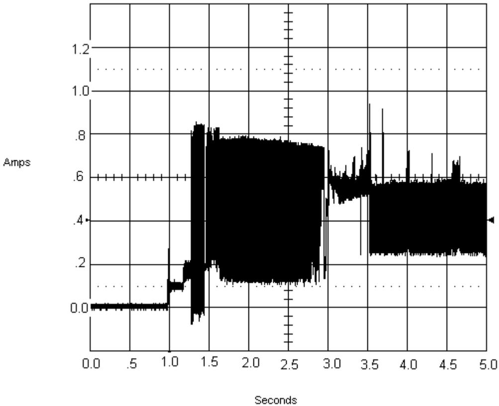
Figure 2. Typical 5V startup and operation current profile
