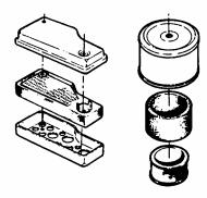
Generally, wash foam-type filters in a dishwashing detergent and water solution. Rinse and wring dry, then saturate with oil and squeeze out excess. Fallure to re-oil this type filter will ruin the engine.
