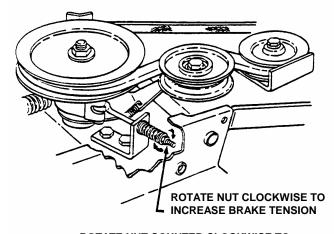
ROTATE NUT COUNTER CLOCKWISE TO DECREASE BRAKE TENSION
