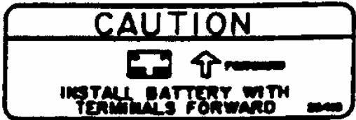
CAUTION! INSTALL BATTERY WITH TERMINALS FORWARD – 2-6415
