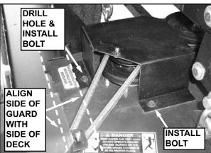
**STEP 8:** Lay supplied pulley guard onto deck. Align hole in front flange with front mounting hole in deck, and secure with one of the two bolts securing original guard. Do not tighten yet.
