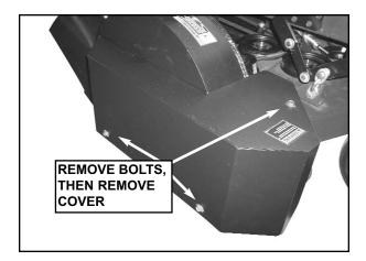
**STEP 6a:** Remove bolts securing impeller pulley cover to blower, and remove cover.
