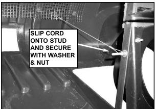
**STEP 17:** Slip looped end of cover support cord onto threaded stud on hose adapter assembly. Secure end of cord with one 3/16" flat washer and 10-32 nyloc nut (not shown). Run nut all the way in on thread, but leave cord loose enough to swivel.
