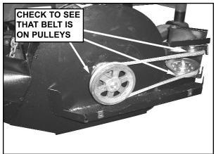
**STEP 6b:** Check to see that blower belt is routed around impeller pulley and idler pulleys after belt is installed onto deck pulley. Then replace cover. Tighten bolts securely. **IMPORTANT:** Never operate any mower without a pulley guard securely in place.
