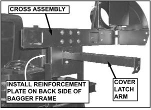
**STEP 14:** Install cross assembly onto bagger frame with four  $3/8-16 \times 3/4$  bolts and hex flange lock nuts, tightening securely. Insert bolts back through bagger frame and into cross assembly.
