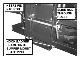
**STEP 13:** Hook bottom of bagger frame onto pins in bottom of bumper mount plate. Then slide locking rod through aligned holes in bagger frame and bumper mount plate, securing with bridge pin.
