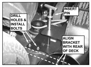
**STEP 7:** Slip tube of locking pin bracket into blower mount, and secure with T-handle pin, making sure pin goes through both upper and lower part of blower mount. Then align base of pin bracket parallel with rear of deck, and, using bracket as a template, drill two 7/16" holes through deck. Insert two 3/8-16 x 1" bolts up through deck and bracket, securing with hex flange nuts. Tighten securely. **IMPORTANT:** Use gloves when working under deck. Sharp blades can cause injury.
