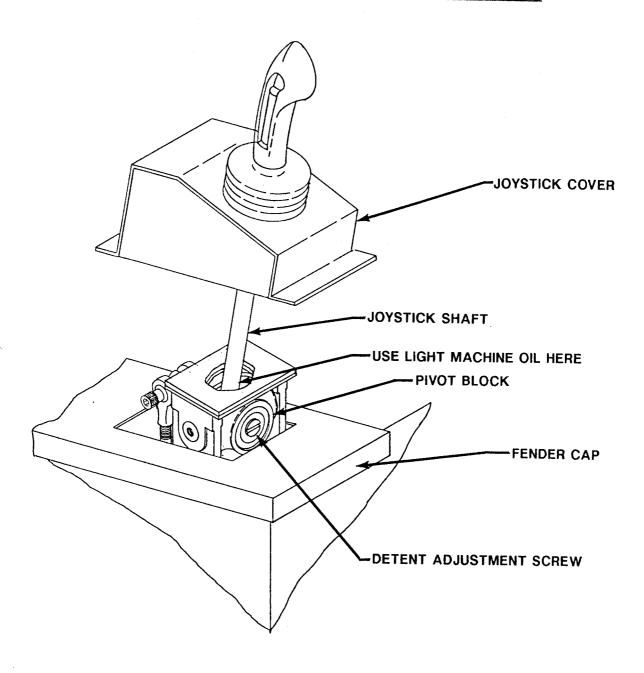
Remove Joystick Cover from Fender Cap.
