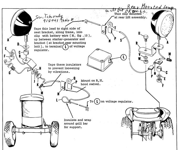
NOTE - As lamp ground is the "return circuit", all lamp and bracket mounting surfaces must be free of paint. Be absolutely certain wires do not rub on moving parts.
