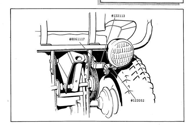
NOTE: To assure good electrical contact, remove the paint from the surfaces of the brackets at points of contact.
