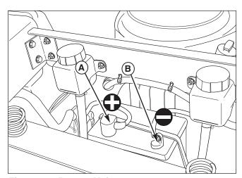
Figure 28. Battery Maintenance
