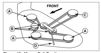
Figure 43. Mower Belt Routing
