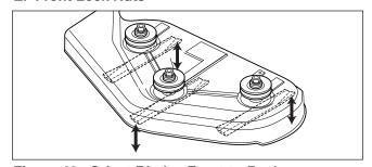
Figure 40. Orient Blades Front-to-Back
