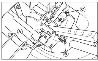
Figure 31. Top Speed Adjustment
