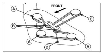
Figure 9. Mower Belt Routing
