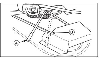
Figure 10. Release Belt Tension A. Belt Tension Release Lever
