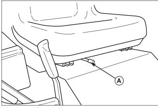
Figure 29. Seat Adjustment A. Adjustment Lever
