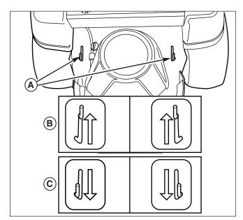
Figure 2. Transmission Release Levers
