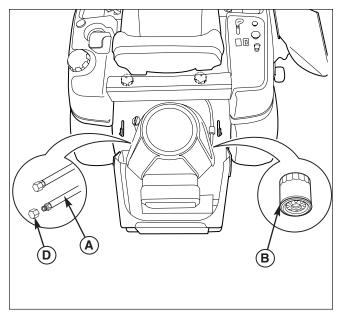
Figure 25. Change Engine Oil & Filter
