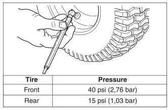
Figure 23. Checking Tire Pressure
