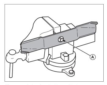
Figure 21. Balancing the Mower Blade A. Nail
