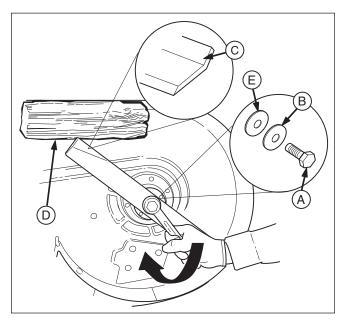
Figure 22. Tightening the Mower Blade for Installation
