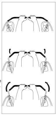
Figure 3. Move Control Levers Gradually
