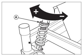
Figure 34. Suspension Adjustment A. Front Shock Adjustment Collar
