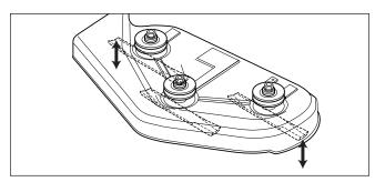
Figure 37. Orient Blades Side-to-Side
