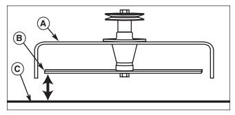
Figure 38. Measure Blade Tips to Ground
