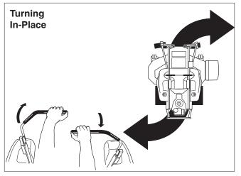
Figure 7. Turning in Place
