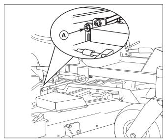
Figure 41. Roller Bar Leveling
