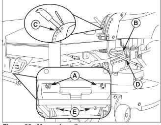
Figure 39. Mower Leveling
