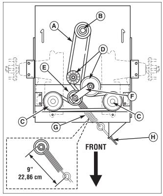
Figure 44. Hydraulic Pump Drive Belt Replacement
