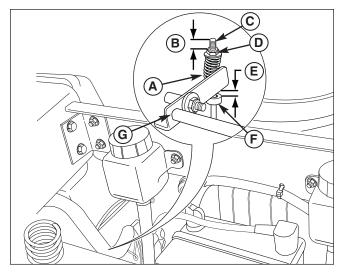
Figure 33. Parking Brake Adjustment
