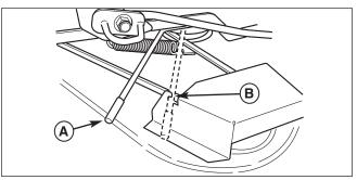
Figure 42. Release Belt Tension
