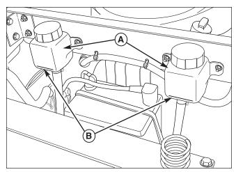
Figure 26. Transmission Oil Reservoirs
