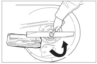
Figure 17. Loosening the Mower Blade for Removal
