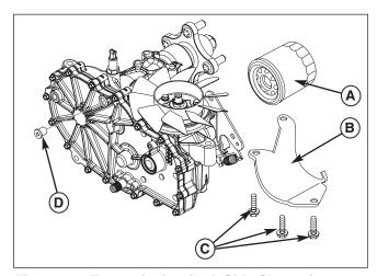
Figure 27. Transmission (Left Side Shown.)
