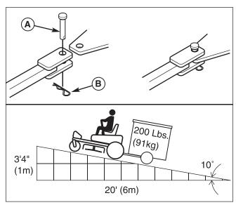
Figure 15. Trailer Weight Recommendations A. Clevis Pin
