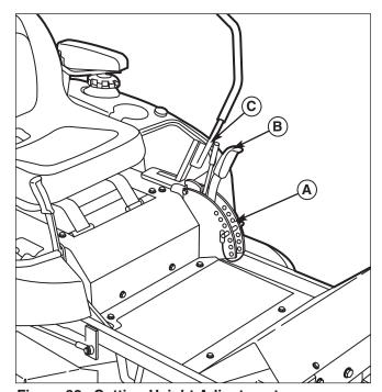
Figure 32. Cutting Height Adjustment
