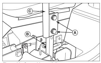
Figure 30. Control Lever Adjustment
