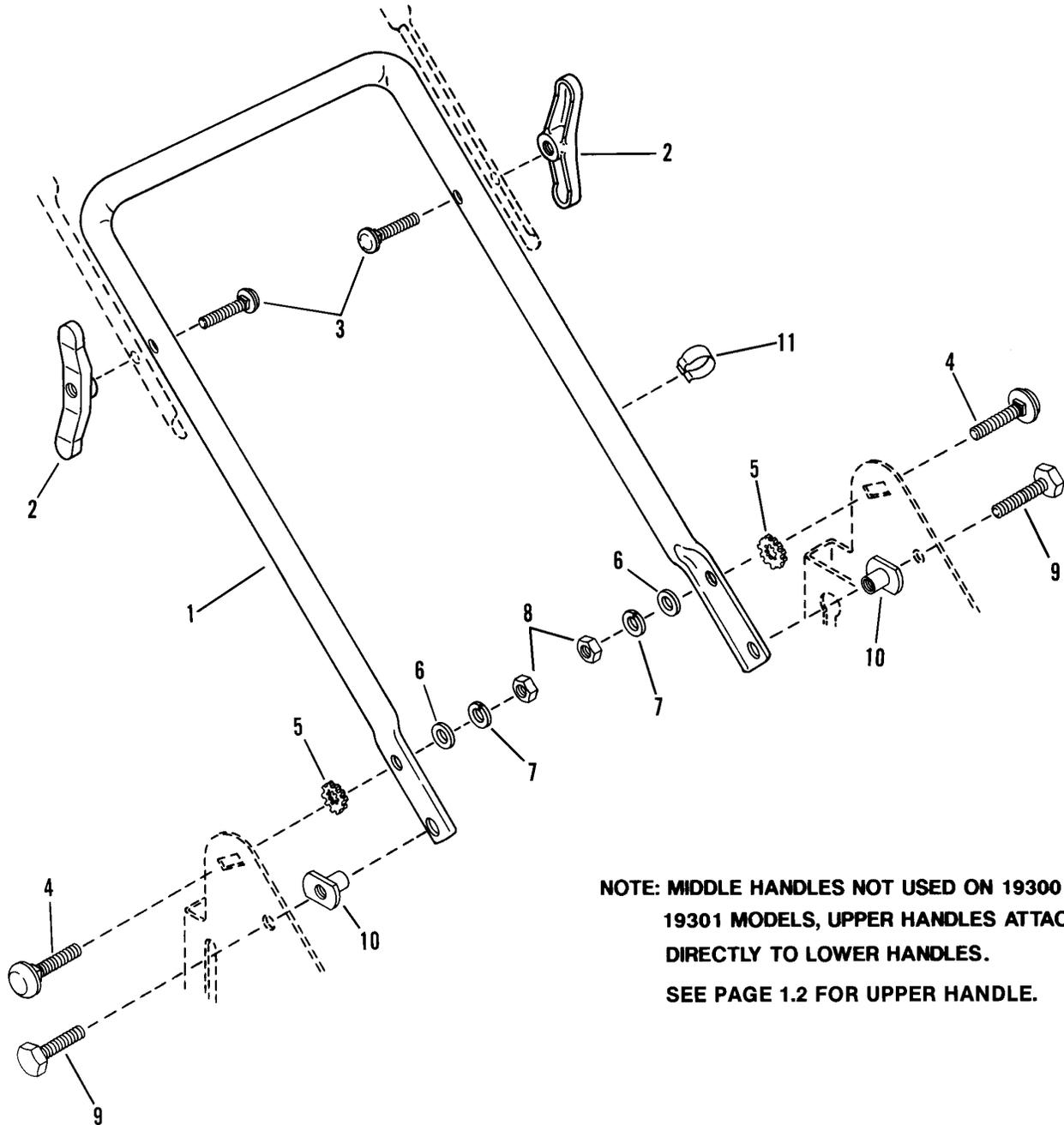
**NOTE: MIDDLE HANDLES NOT USED ON 19300 & 19301 MODELS, UPPER HANDLES ATTACH DIRECTLY TO LOWER HANDLES. SEE PAGE 1.2 FOR UPPER HANDLE.**
