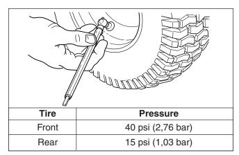
Figure 20. Checking Tire Pressure
