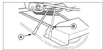
Figure 37. Release Belt Tension
