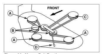
Figure 36. Mower Belt Routing
