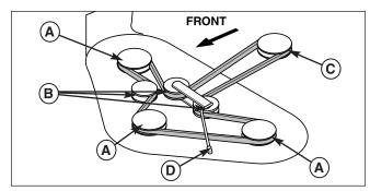
Figure 9. Mower Belt Routing
