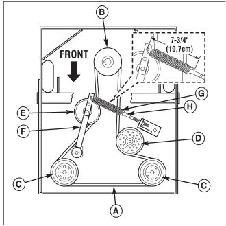
Figure 38. Hydraulic Pump Drive Belt Replacement (Shown from Below)
