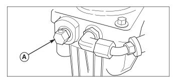
Figure 2. Transmission Release Valves
