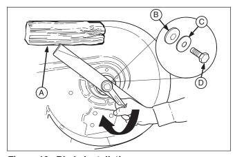
Figure 19. Blade Installation
