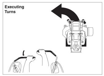
Figure 6. Turning Around a Corner
