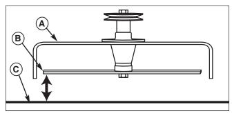
Figure 32. Measure Blade Tips to Ground
