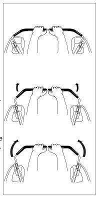
Figure 3. Move Control Levers Gradually
