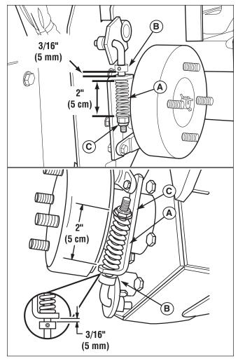
Figure 27. Parking Brake Adjustment
