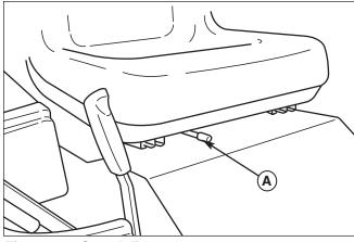
Figure 23. Seat Adjustment A. Adjustment Lever
