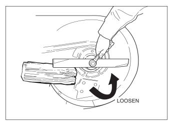
Figure 17. Blade Removal
