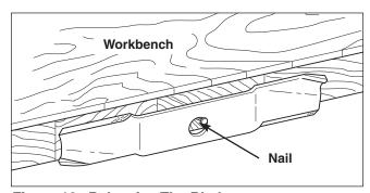
Figure 18. Balancing The Blade
