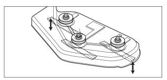
Figure 31. Orient Blades Side-to-Side
