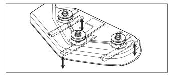
Figure 34. Orient Blades Front-to-Back
