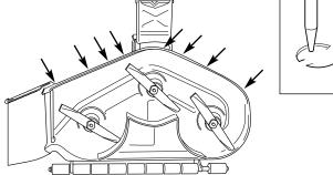
**1** Step One — Remove the mower deck from the tractor. Locate the eight knock-outs as shown by the arrows in the illustration above. Knock these out carefully with a punch as shown in the inset above and twist out.
