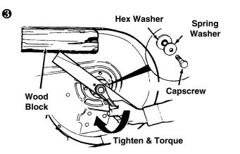
Step Three — Install the Mulching Blades with tabs pointing up towards the deck. Use a wooden block to prevent blade rotation. *Torque each blade mounting capscrew to 50-70 ft. lbs. (67-95 N.m.)*
