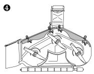
• Step Four — Position the baffle so the discharge edge contacts the stone guard. Hold the baffle in position with clamps as shown.
