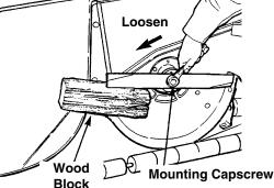
Step Two — Remove the standard blades using a wood block to hold blades in position while removing the mounting capscrew as shown above.
