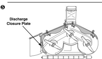
**6** Step Five — Position the Discharge Closure Plate at the discharge opening of the mower deck, inserting the tab into the baffle. Hold the plate in position with clamps as shown.
