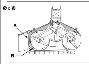
**9** Step Nine— Attach the closure plate with phillips screws, lockwashers, and nuts as shown above. ("A" is inserted from the top of the deck. "B" is inserted from the bottom of the closure plate/deck.) Tighten the nuts securely and remove the clamps.
