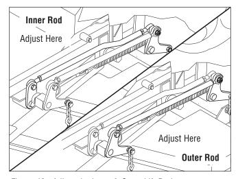
Figure 42. Adjust the Inner & Outer Lift Rods
