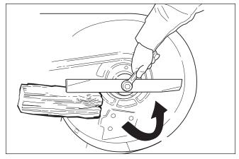
Figure 26. Loosening the Mower Blade for Removal
