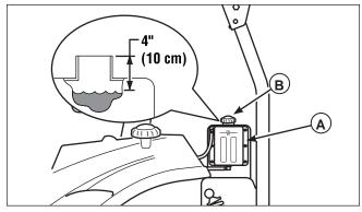
Figure 19. Checking Hydraulic Oil Level
