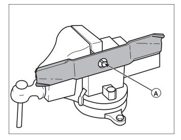
Figure 30. Balancing the Mower Blade A. Nail
