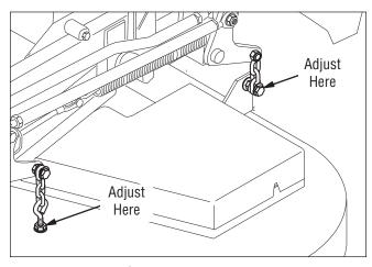
Figure 44. Hanger Chain Adjustment
