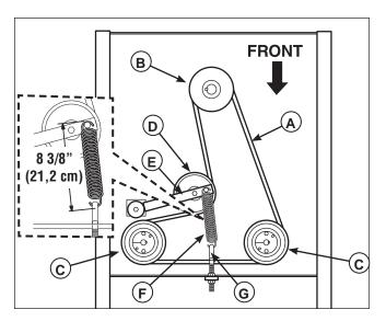
Figure 38. Hydraulic Pump Drive Belt Replacement
