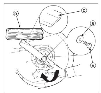
Figure 31. Tightening the Mower Blade for Installation
