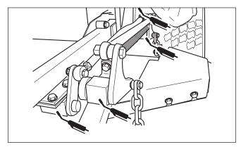
Figure 23. Deck Lift Linkage Pivots
