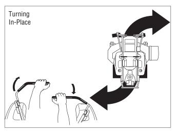
Figure 11. Turning in Place
