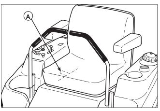
Figure 3. Seat Adjustment A. Seat Adjustment Lever
