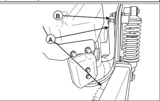
Figure 18. Engine Oil Drain
