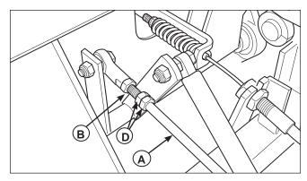
Figure 35. Neutral Adjustment (RH side shown)
