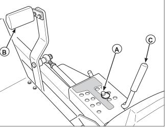
Figure 5. Mowing Height Adjustment A. Cutting Height Adjustment Pin
