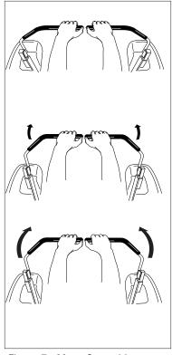
Figure 7. Move Control Levers
