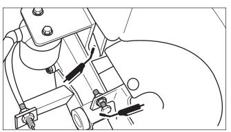
Figure 24. Suspension & Deck Lift Pivots
