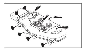
Figure 21. Deck Lubrication
