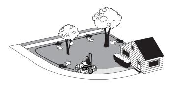
Where possible, make one or two passes around the outside of the area discharging the grass INTO the lawn to keep the cut grass off fences and walks.
