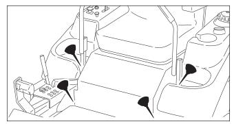
Figure 22. Control Handle Pivots & Seat Plate Pivots
