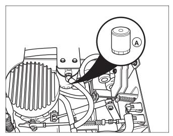
Figure 20. Change Hydraulic Oil Filter A. Hydraulic Oil Filter
