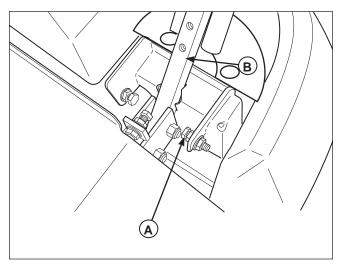
Figure 34. Top Speed Adjustment A. Top Speed Adjustment Bolt
