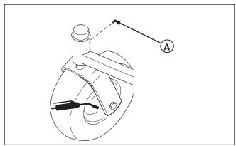
Figure 25. Front Caster & Wheel A. 1/4-28 Bolt
