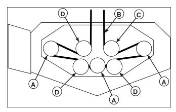
Figure 47. Mower PTO Belt Routing
