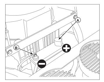
Figure 32. Battery Compartment A. Positive (+) Cable & Terminal B. Negative (-) Cable & Terminal
