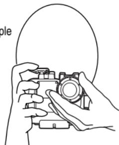
**CAUTION** : • Do not exert excessive force onto the lens window or the lens ring.
