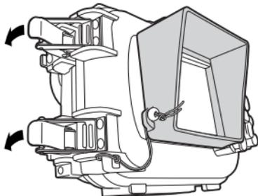
**⚠ CAUTION :** • Seal the Case by turning both buckle lock levers down in arrow direction. When one of the buckles is left open, the Case will not be sealed and water leakage will be caused.
