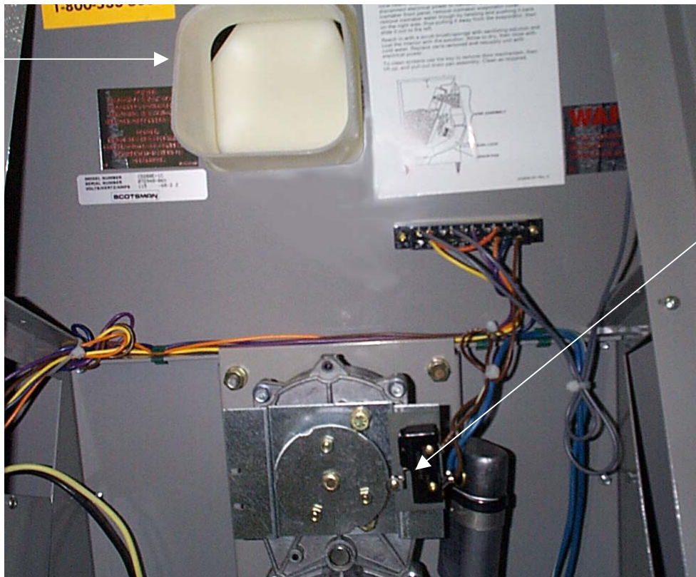
Correct positions of cam and rotor at rest.
