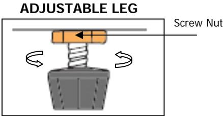
The wine chiller has adjustable legs on the front of the unit. The legs are preset by the factory to a specific height with a screw nut for proper height. Please make sure this screw nut is in place at all times. Do not remove it under any circumstances.
