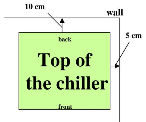
**NOTE: THE SPACING IS NECESSARY FOR PROPER VENTILATION**
