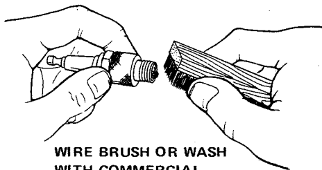
Figure 21. Clean or Replace Spark Plug (Yearly Care)
