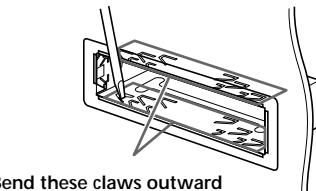
Bend these claws outward for a tight fit, if necessary.
