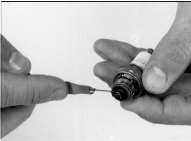
6. Check plug gap with a wire feeler gauge, gap should be 0.76 mm (0.030 in.)
