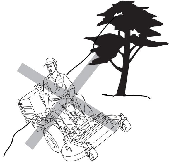
Figure 4-8 Improper Operation on a Slope
