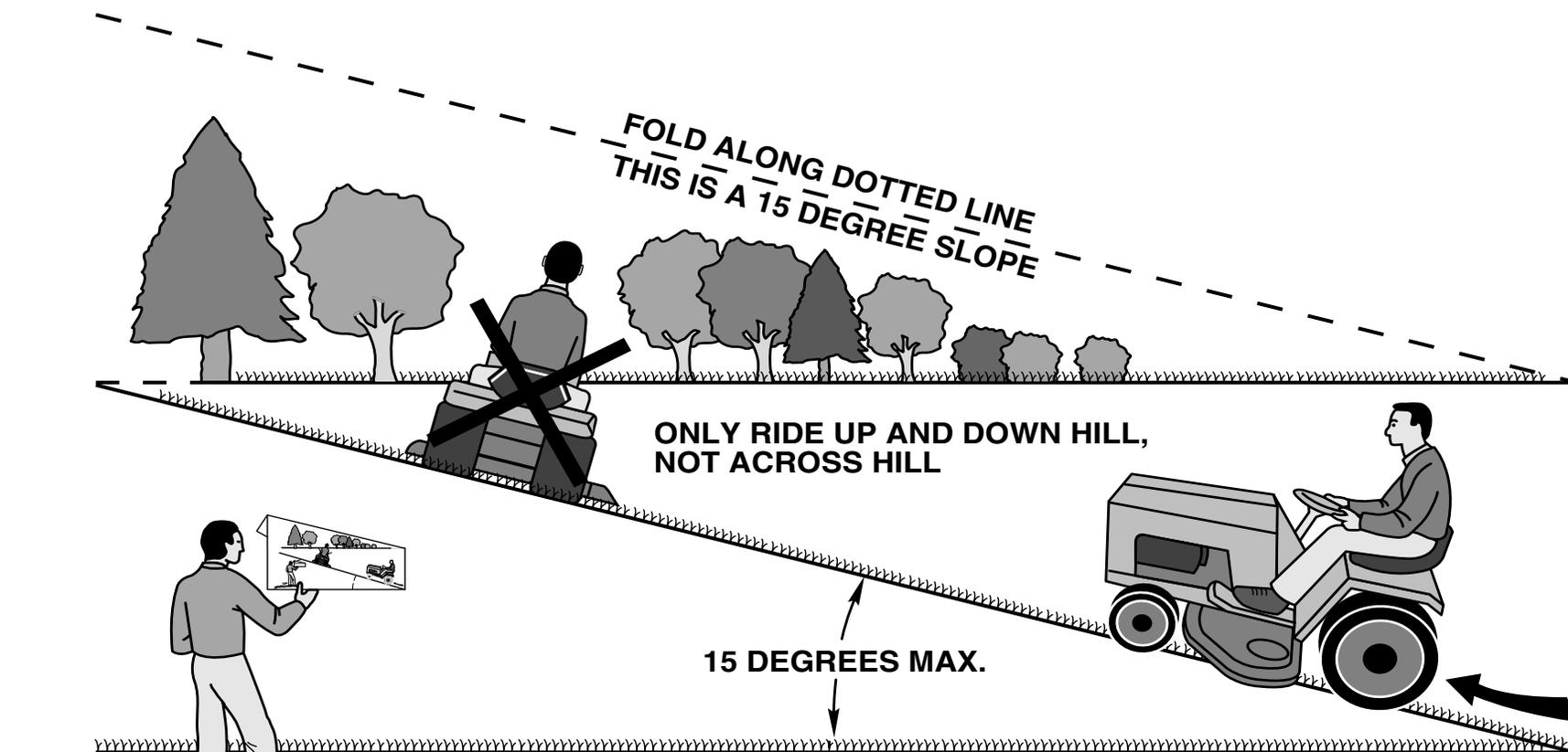
**WARNING:** To avoid serious injury, operate your tractor up and down the face of slopes, never across the face. Do not mow slopes greater than 15 degrees. Make turns gradually to prevent tipping or loss of control. Exercise extreme caution when changing direction on slopes.
