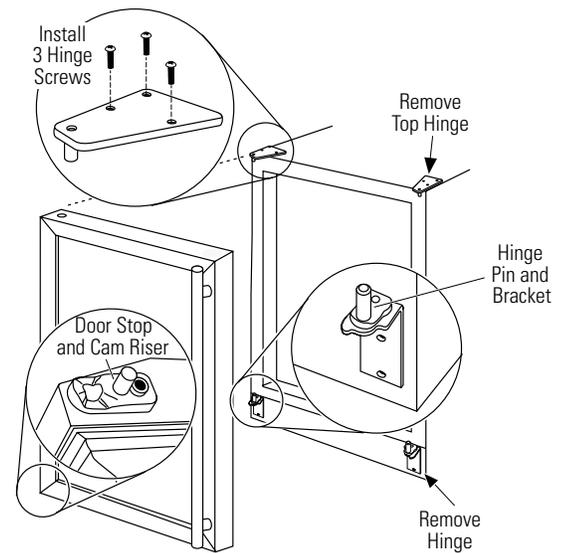
3. Place the door onto the bottom case hinge.
