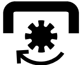
ATTACHMENT CLUTCH ENGAGED
