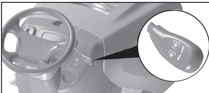
(☞) ATTACHMENT CLUTCH SWITCH "DISENGAGED"
