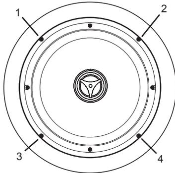
Tighten all four of the mounting screws in the same manner until the speaker is properly aligned and held tight to the ceiling surface. **Caution: Do not over tighten!**
