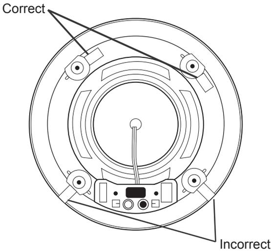
With the grill removed, place the speaker in the ceiling opening. Make sure that the speaker wire is not hanging against the speaker where it can vibrate and rattle as the speaker reproduces your audio program.
