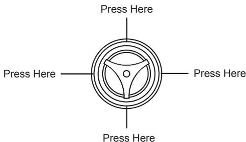
Using gentle pressure, swivel the tweeter to aim the axis of the tweeter toward the listening area. You can use a piece of music with a solid center-imaged vocalist to assist in correctly aiming the tweeter. When the tweeters are properly aligned, you will hear a coherent and stable center image from your listening position. Usually, it is sufficient to aim the tweeter only, as it handles the frequencies that control the direction of individual sounds in your audio program material.
