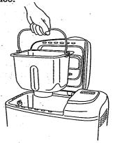
If the pan does not snap securely into place, remove bread pan. Wearing oven mitts, place fingers behind bread pan clips and gently pull away from oven wall. Insert bread pan again.
