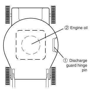
(1) Spray lubricant 2 See "ENGINE" in Maintenance section.
