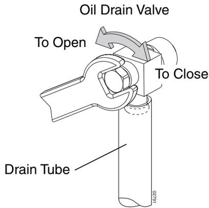
4. After oil has drained completely, close the drain valve turning clockwise. Use the 7/16" (11mm) wrench to apply a small amount of torque to keep it closed. Do not over tighten.
