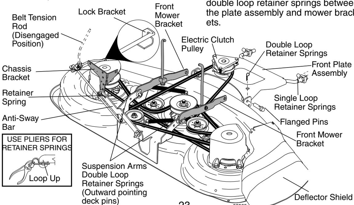
**NOTE:** To assist in locating hole in flanged pin, the hole in pin is inline with notch on head of pin. If necessary, move mower side-to-side to give space between plate and mower brackets.
