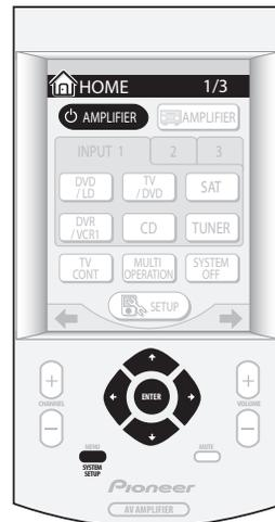
An on-screen display (OSD) appears on your TV. Use the **↑/↓/←/→** hard keys and **ENTER** on the remote control to navigate through the screens and select menu items.
