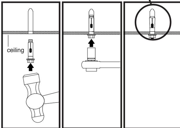
**STEP1:** Hammer in concrete anchor.
