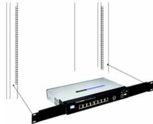
Figure 3-3: Mount the Switch in the Rack
