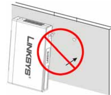
Figure 3-5: Incorrect Wall-Mount Orientation (Vertical)
