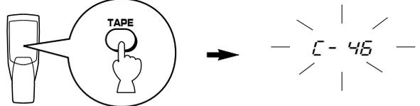
You can select any of four tape lengths by pressing the **TAPE** button.
