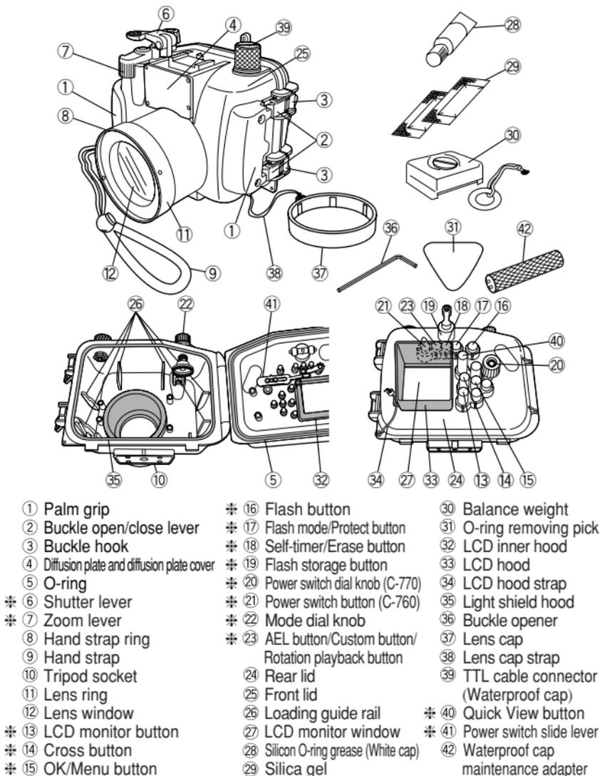
**Note :** The Case operation parts marked by\* corresponds to the operation parts of the digital camera. When the operation parts of the Case are operated, the corresponding functions of the digital camera will operate. For details of the functions, refer to the instruction manual for the digital camera.
