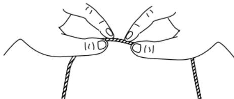
Using a clean cloth free of fibers, dirt, etc., a piece of lint-free tissue paper or a soft toothbrush, remove any foreign matter attached to the grooves of the O-rings. Also remove sand and dirt particles attached to the O-ring contact surfaces on the case.
