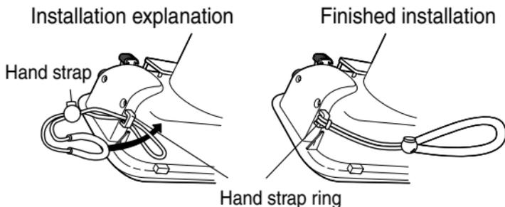
**CAUTION** : Please install the strap correctly as shown above. OLYMPUS CORPORATION shall bear no responsibility for damage etc. caused by dropping the Case because of incorrect installation of the strap.
