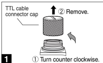
**1** Remove the TTL cable connector cap from this case.
