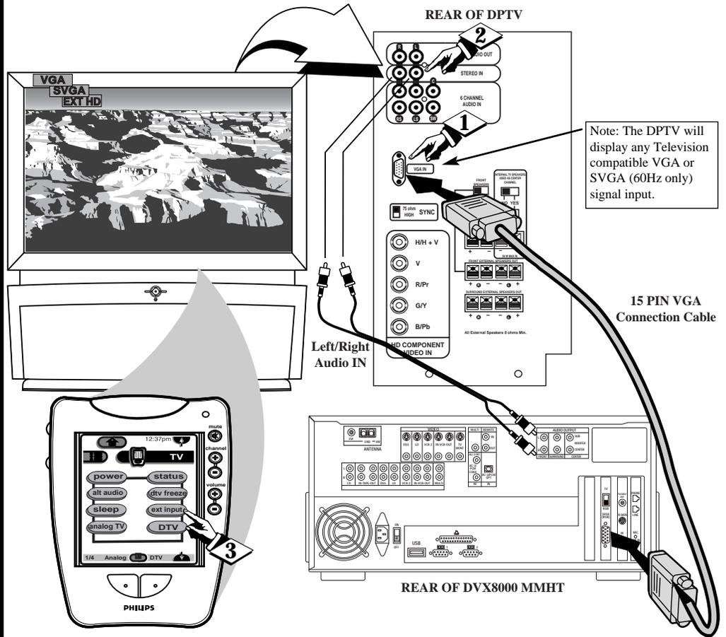
Note: The DPTV will display any Television compatible VGA or SVGA (60Hz only) signal input.
