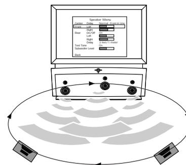
Test Tone signal circulates through the speaker system in a clockwise direction, and is meant to be used with the adjustable Speaker Menu "barscale" controls (such as Front Speaker Left/Right and Rear Speaker Left/Right). Once turned On, the Test Tone will continue to circulate through the Front and Rear speakers (even when other sound controls are selected, such as Subwoofer, which are not adjustable within the Test Tone mode.)
