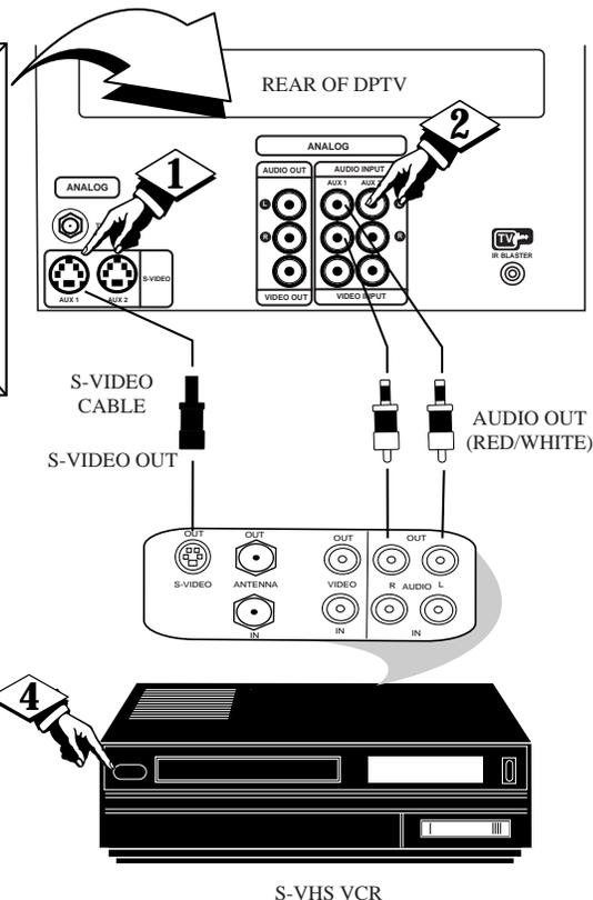
**NOTE:** A CD-i (Compact Disc Interactive) player, Video Game, or other S-VIDEO accessory can be hooked up to the DPTV using this type of connection. Please be aware that such video sources, which show a constant non-moving pattern on the DPTV screen, can cause picture tube damage. When not in use turn your video accessories OFF. Also, regularly alternate the use of video sources with normal TV program viewing.
