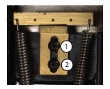
For HP Specials equipped with the Floyd Rose licensed tremolo, we have included another Peavey innovation called the Lok Block. By loosening the screws (#1 & 2 at left) with the included hex wrench and sliding the Block back and forth, you can choose between a floating style tremolo or a more traditional tremolo that only has downward movement. With the Lok Block, you can choose for yourself!
