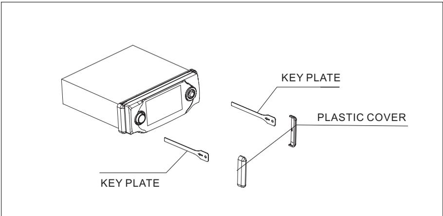
If you want to take CHASSIS out of the SLIDE BRACKET HOUSING, first remove the PLASTIC COVER of the both sides away, then insert the two KEY PLATE into left and right side of chassis as above illustration.
