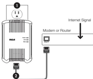
1. Plug one of the HDP50 units into an electrical outlet near your modem. The **Power** indicator on the front of the adapter illuminates.
