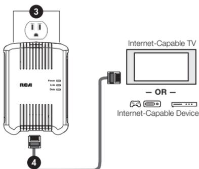
3. Plug the other HDP50 unit into an electrical outlet near your TV or other home entertainment device that is Internet-capable. The **Power** indicator on the front of the adapter illuminates.
